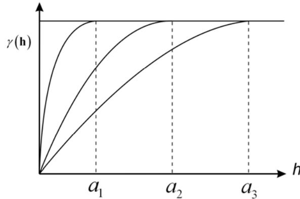
**Figure 1:** Three variograms calculated at different directions show the geometric anisotropy in depositional setting.
